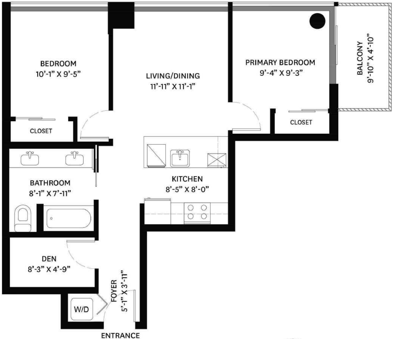
MAIN FLOOR PLAN Ceiling Height 8'-0"
